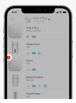
When the range extender detects a malfunction (for example, there is no external power supply), the Ajax app displays a badge with counter in the upper left corner of the device icon.
