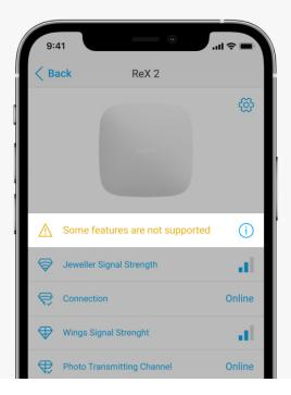
ReX 2 can notify about malfunctions, if any. **Malfunctions** field is available in **Device States**. Clicking on i opens the list of all malfunctions. Note that the field is displayed if a malfunction is detected.
